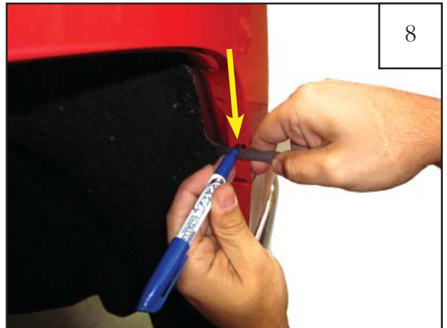
Remove the flare. At the marked locations made in Step 6, measure inward 22mm from the edge of the fender and mark with grease pencil or marker. These are the marks to be drilled.
